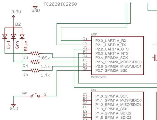
Figure 3. LED and pushbutton schematic.
