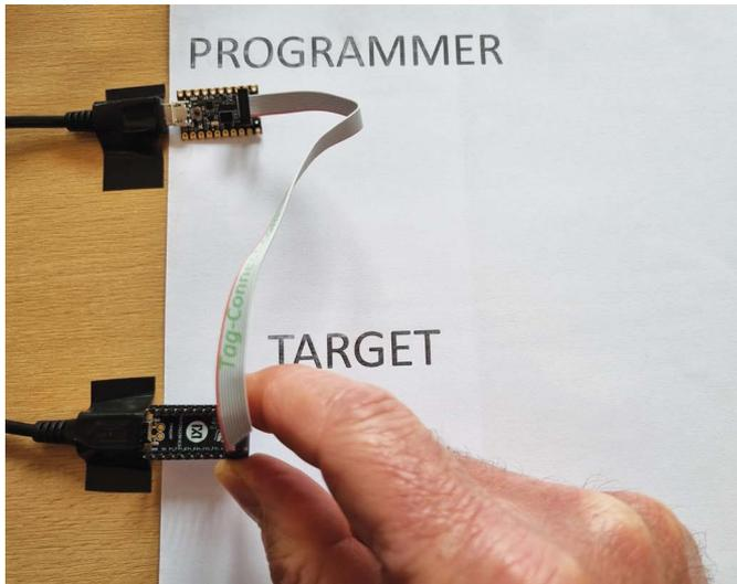
Figure 9. Connecting the programmer to the target.
